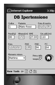
Figure 4: A part of the graphical user interface of the Homey database, and its reduced version suited for PDA displays. The small telephone icon indicates that the data entry was performed by the patient himself, dialling into the automatic dialogue system. The most frequently used input fields will be voice-enabled by the multi-modal technology explained in the article.
